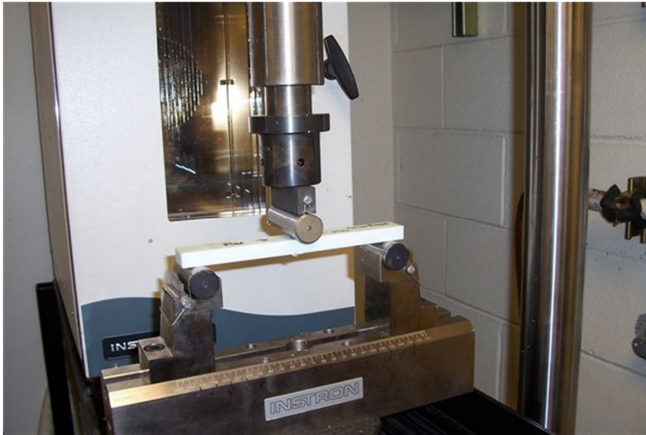
ASTM D790 - Flexural Testing – 3 Point Flex Strength of adhesive joints
